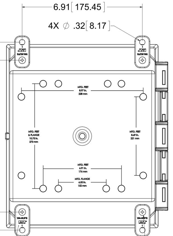
(4) EACH #10-32 BRASS INSERTS, AND 316 STAINLESS STEEL FLANGE AND FEET SCREWS
