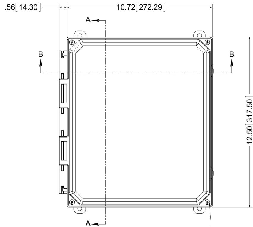
(4) EACH #10-32 BRASS INSERTS, AND 316 STAINLESS STEEL CAPTIVE COVER SCREWS WITH RETAINING O-RING
