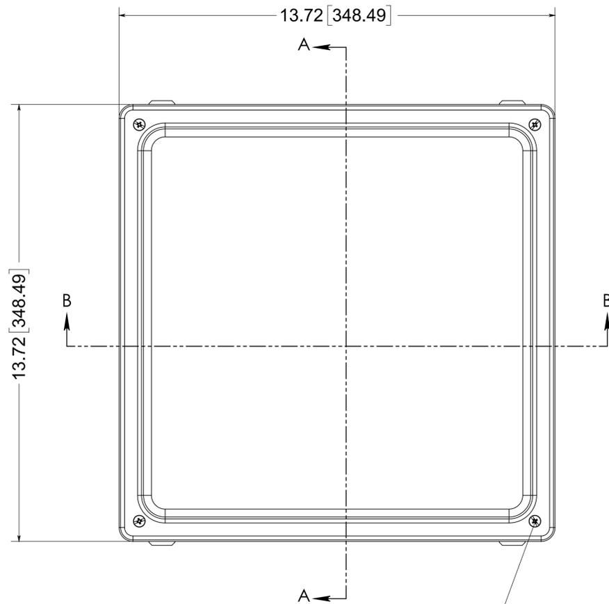
(4) EACH #10-32 BRASS INSERTS AND 316 STAINLESS STEEL CAPTIVE COVER SCREWS WITH RETAINING O-RING
