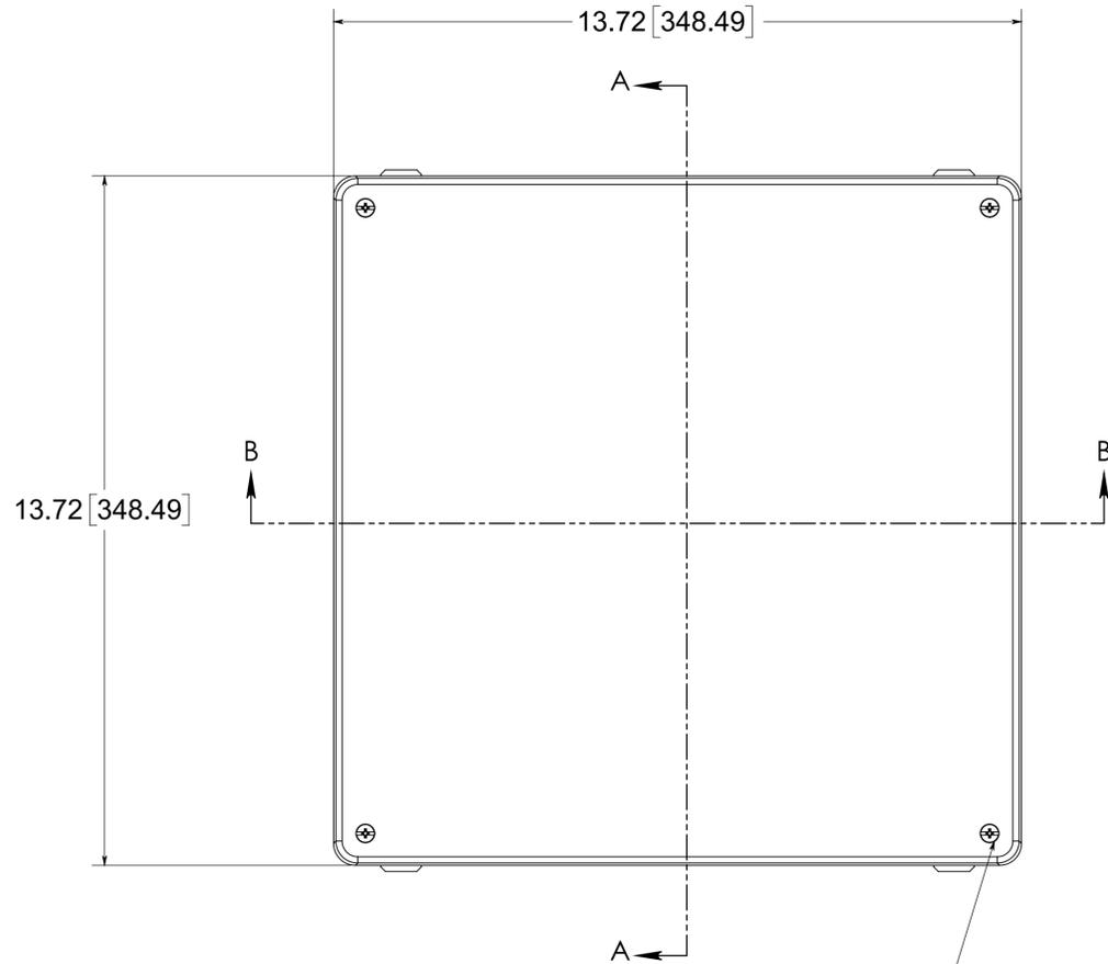
(4) EACH #10-32 BRASS INSERTS AND 316 STAINLESS STEEL CAPTIVE COVER SCREWS WITH RETAINING O-RING
