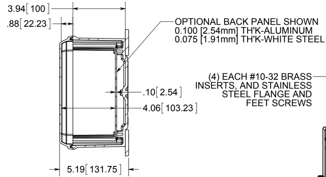
(4) EACH #10-32 BRASS INSERTS, AND STAINLESS STEEL FLANGE AND FEET SCREWS
