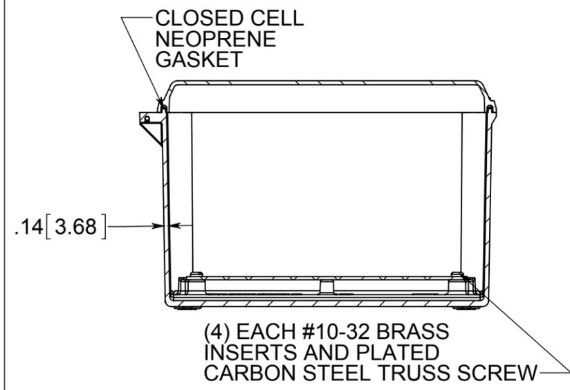
(4) EACH #10-32 BRASS INSERTS AND PLATED CARBON STEEL TRUSS SCREW
