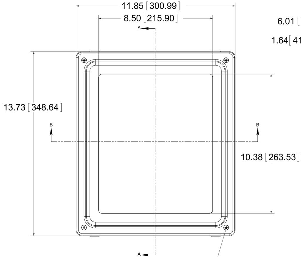
(4) EACH #10-32 BRASS INSERTS AND STAINLESS STEEL CAPTIVE COVER SCREWS WITH RETAINING O-RING
