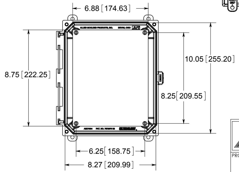
STAINLESS STEEL LOCKABLE SNAP LATCH LOCATED ON CENTER
