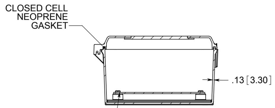
(4) EACH #10-32 BRASS INSERTS AND PLATED CARBON STEEL SCREWS
