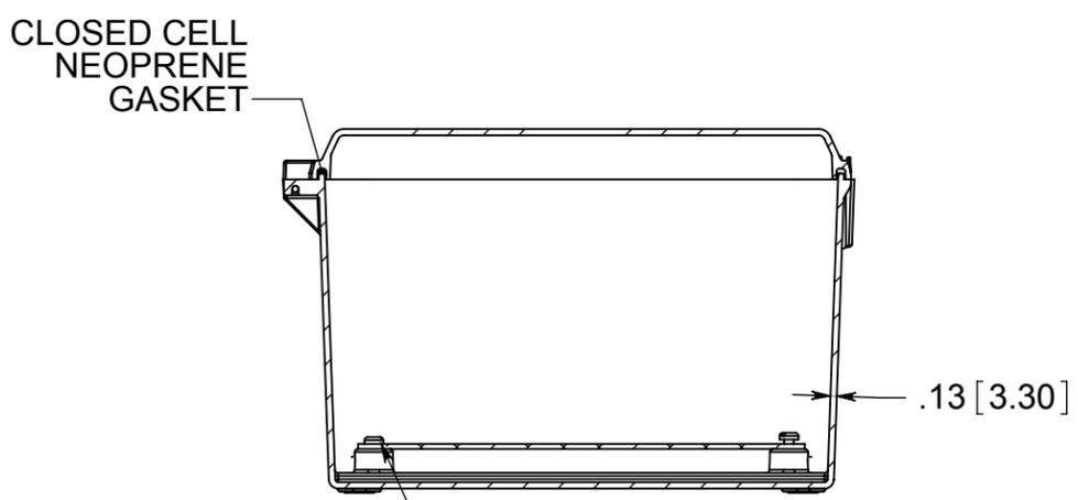
(4) EACH #10-32 BRASS INSERTS AND PLATED CARBON STEEL SCREWS
