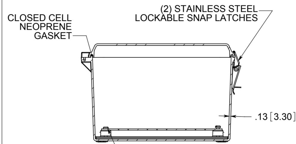
(4) EACH #10-32 BRASS INSERTS AND PLATED CARBON STEEL SCREWS
