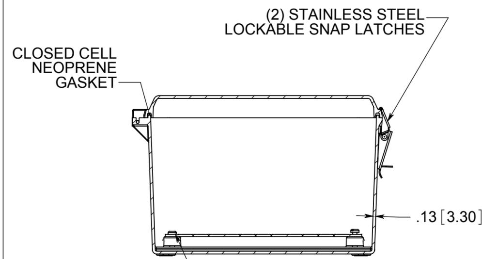
(4) EACH #10-32 BRASS INSERTS AND PLATED CARBON STEEL SCREWS
