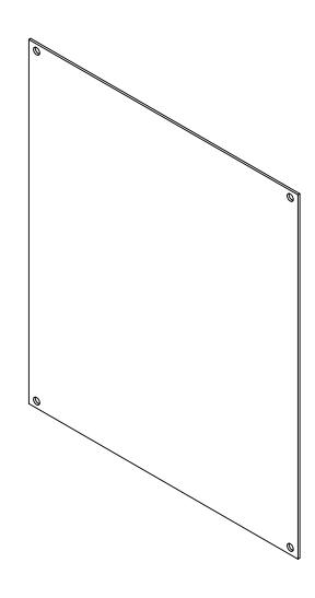
Galvannealed 14 Gauge Steel
