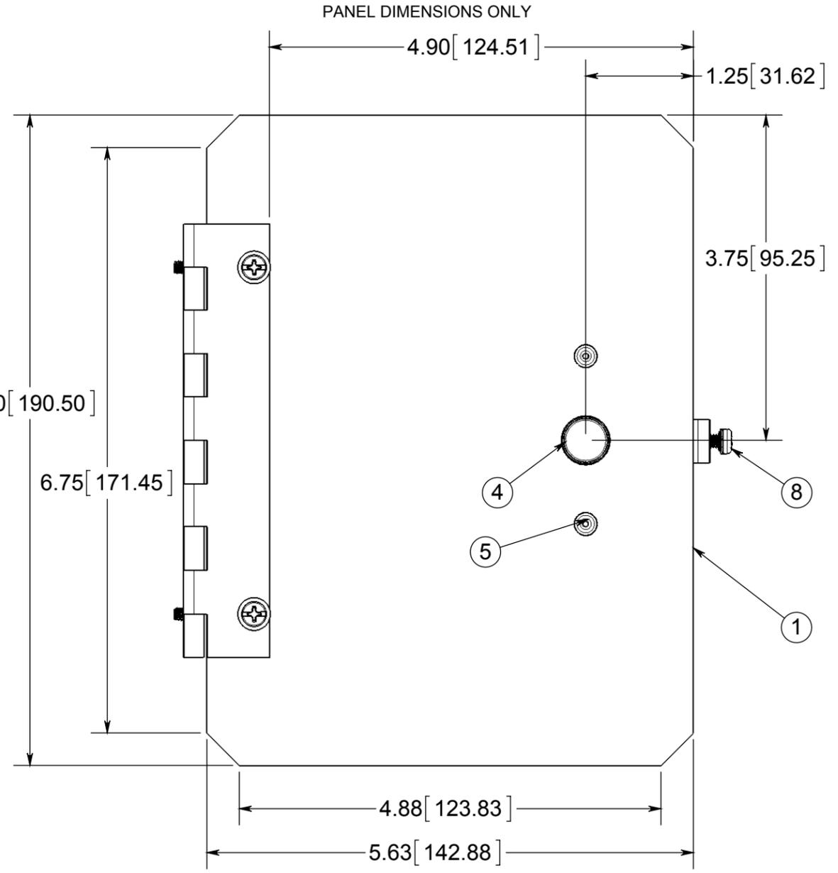
NOT ALL PARTS OF THE HFP ASSEMBLY KIT ARE SHOWN, ONLY THE PARTS USED IN THE FLUSH INSTALLATION OF THE PANEL. FOLLOW INSTALLATION INSTRUCTIONS INCLUDED IN THE KIT FOR THE OPTIONAL PANEL MOUNTING.
