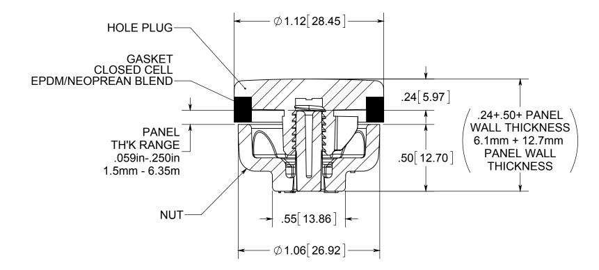
PLUGGED HOLE DIA RANGE: .625in-.812in 15.875mm-20.62mm
