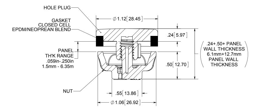
PLUGGED HOLE DIA RANGE: .500in-.624in 12.7mm-15.85mm
