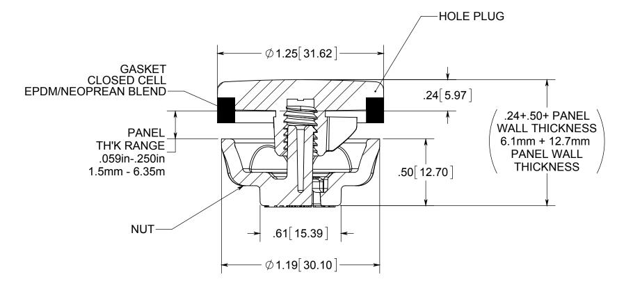
PLUGGED HOLE DIA RANGE: .812in-.937in 20.62mm-23.80mm
