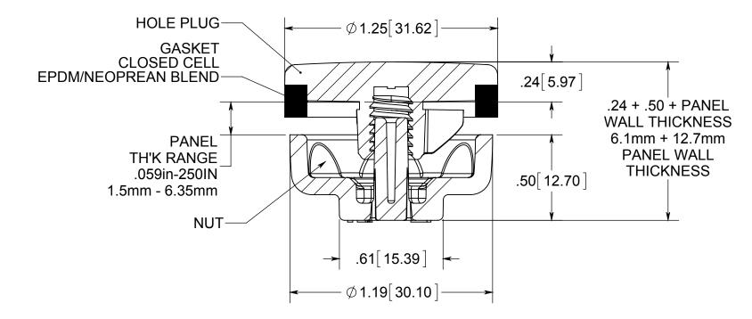
PLUGGED HOLE DIA RANGE: .812in-.937in 20.62mm-23.80mm
