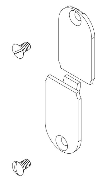
NOTES: 1.) COVER PLATE MATERIAL: BRASS, COVER PLATE MOUNTING SCREW MATERIAL: BRASS 2.) WHEN USED WITH FB-4 FLOOR BOX IT IS UL LISTED, FLOOR BOX MEETS UL514C SCRUB WATER EXCLUSION TEST
