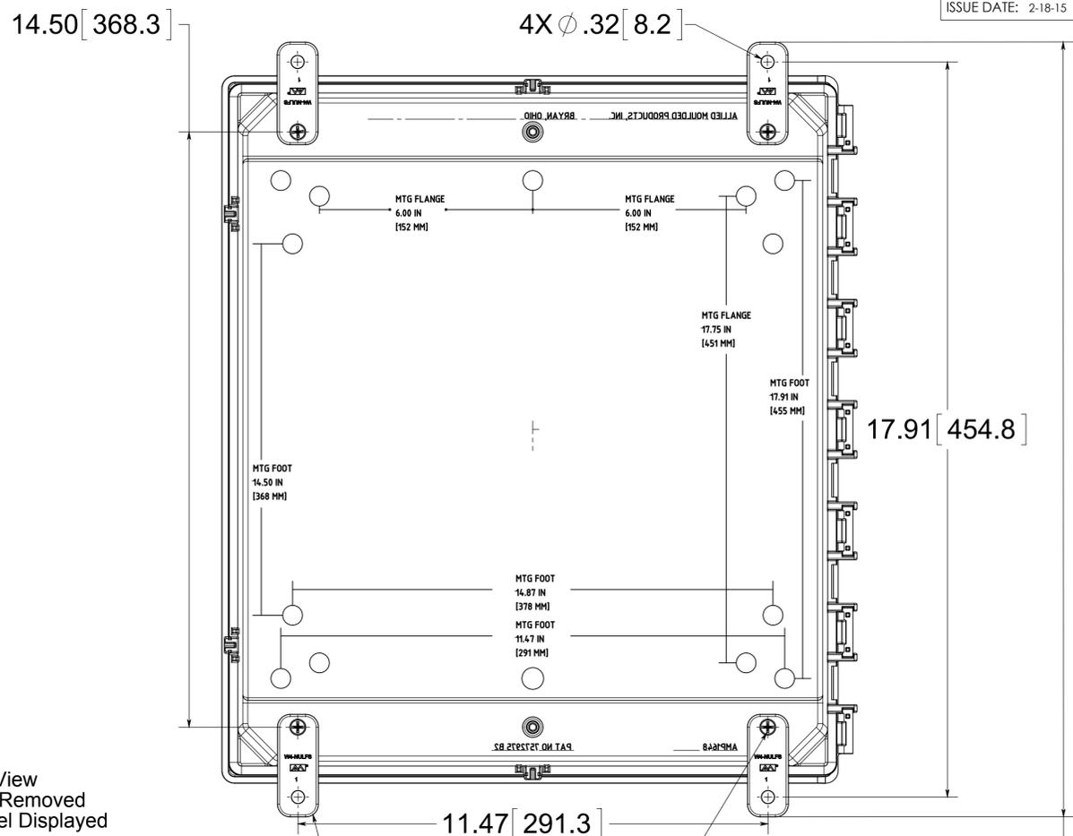
4X #10-32 Brass Inserts and Plated Carbon Steel Truss Screw
