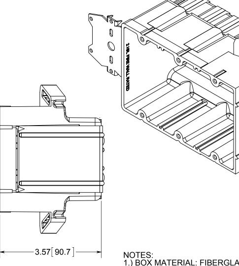
1.) BOX MATERIAL: FIBERGLASS REINFORCED POLYESTER, BRACKET MATERIAL: GALVANIZED STEEL.
