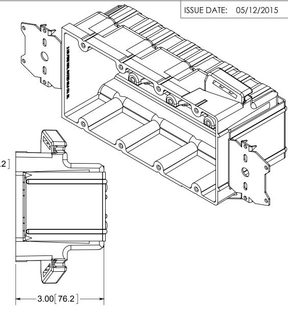
NOTES: 1.) BOX MATERIAL: FIBERGLASS REINFORCED POLYESTER, BRACKET MATERIAL: GALVANIZED
