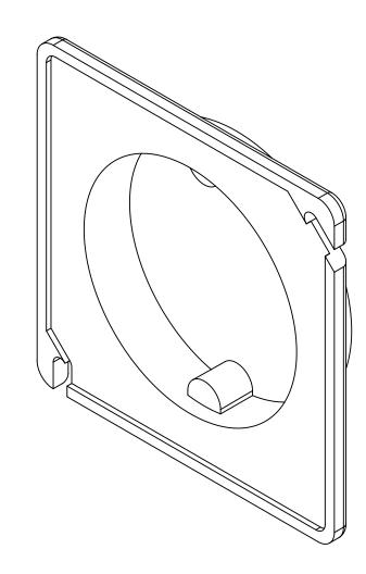
NOTES: 1.) BOX MATERIAL: FIBERGLASS REINFORCED POLYESTER 2.) USE WITH SERIES 9339, 9342, AND 9343 ONLY 3.) REDUCES TO 3/0 OUTLET
