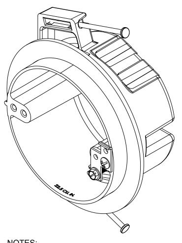
1.) BOX MATERIAL: FIBERGLASS REINFORCED POLYESTER, NAIL MATERIAL: PLATED CARBON STEEL, SPEED KLAMP MATERIAL: PVC, VAPOR SEAL MATERIAL: POLYURETHANE, GROUND MATERIAL: GALVANIZED STEEL, GROUND MOUNTING SCREW MATERIAL: ZINC PLATED STEEL, GROUND SCREW MATERIAL: GREEN ZINC PLATED STEEL
