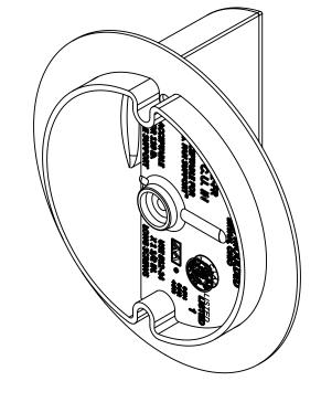
1.) BOX MATERIAL: FIBERGLAS REINFORCED POLYESTER, MOUNTING HARDWARE MATERIAL: ZINC PLATED STEEL
