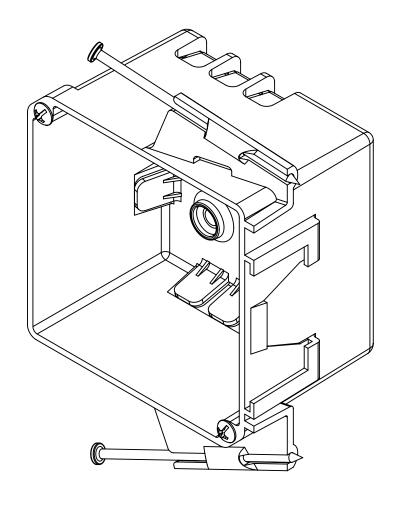
NOTES: 1.) BOX MATERIAL:POLYCARBONATE, NAIL MATERIAL: PLATED CARBON STEEL, SCREW MATERIAL: ZINC PLATED STEEL 2.) UL LISTED WITH 2 HOUR FIRE RATING FOR WALL
