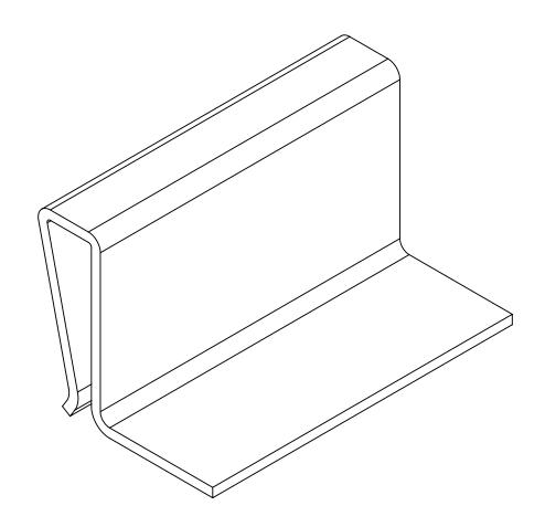
1.) PANEL STOP MATERIAL: NYLON 2.) PANEL STOP TO SQUARE UP BOX IN MISALIGNED WALLS
