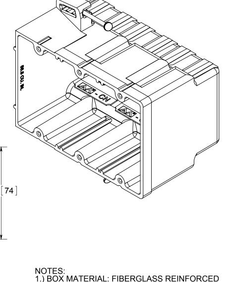
1.) BOX MATERIAL: FIBERGLASS REINFORCED POLYESTER, NAIL MATERIAL: PLATED CARBON STEEL, WIRE CLAMP MATERIAL: GALVANIZED STEEL, WIRE CLAMP SCREW MATERIAL: ZINC PLATED STEEL
